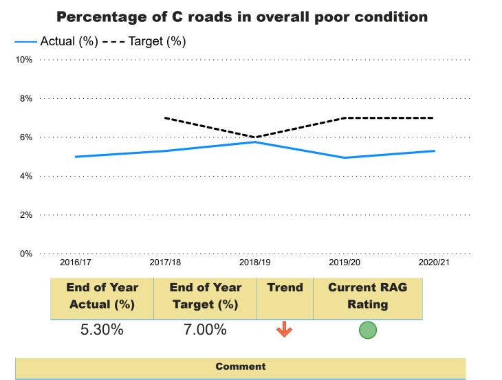
Welsh Government Scanner Data received in September 2020 shows an increase in the length of 'C' roads deemed to be in a poor conditions. This is a result of the annual level of investment in the highway network being below the level required to maintain a steady state, despite any reduction in the usage during the initial stages of the pandemic. However, national data continues to show the roads within Flintshire have the lowest proportion in poor condition.
